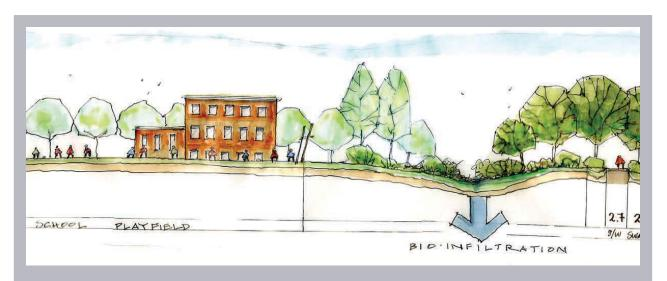
Bioswales (bio-infiltration areas) promote absorption and infiltration of stormwater runoff in urban areas
