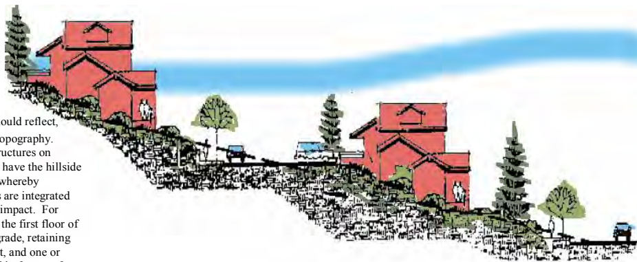
A multiple family development that steps up the hillside to match the topography and reduce the impact on neighbouring buildings
