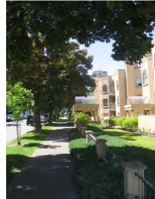
This development contributes to the vitality of the street through the use of appropriate building height, picture windows, balconies, gardens, and a transparent, low-level fence at the property line.
