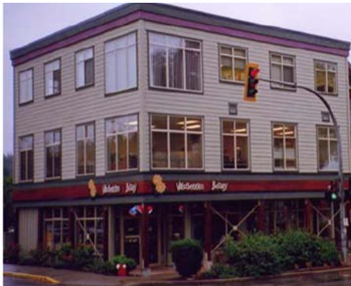
✓ Ground level should provide pedestrian interest; upper storeys should be setback or distinguished by architectural features.
