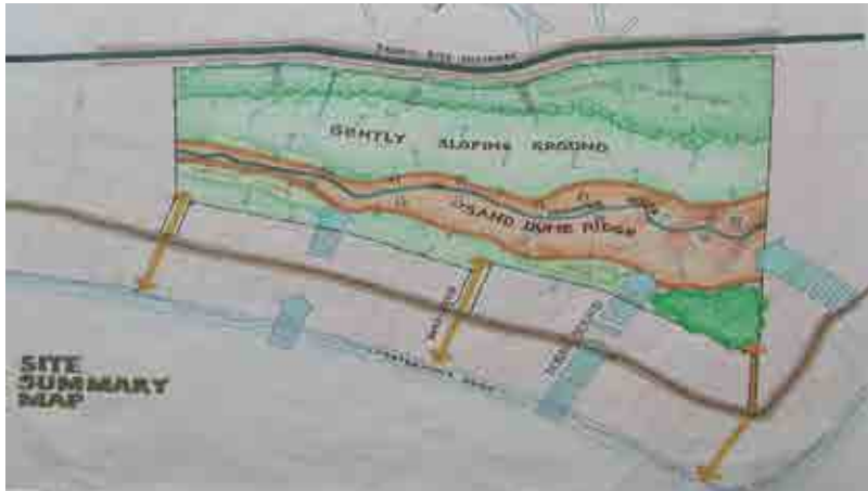
Figure 17: Stormwater management zones. Infiltration will be the primary means of stormwater management in the heart of the site.
