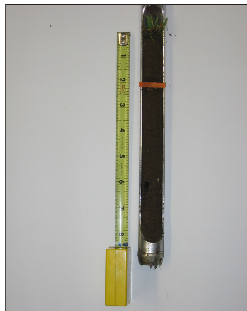
Figure 4. Soil probe that demonstrates separating the top 2 inches of soil from the lower 6 to 8 inches.
