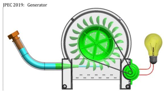
The objective is to make as much electrical energy as possible over a 30 second test using a hand-made generator/turbine and a 5 gallon pail of water which is positioned 10 metres above ground level.
