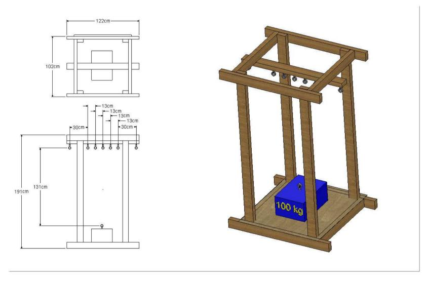
Figure 1: JPEC 2009 block and tackle testing frame
