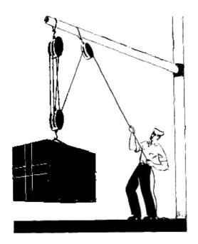
A block and tackle is a system of two or more pulleys with a rope or cable threaded between them, usually used to lift or pull heavy loads. Although used in many situations, they are especially common on boats and sailing ships, where motorised aids are usually not available and the task must be performed manually.
