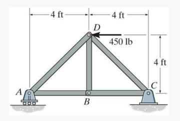
Given: Loads as shown on the trussFind: The forces in each member of the truss.
