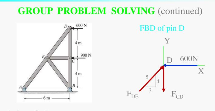
Analyzing pin D:  $\rightarrow + \sum F_X = F_{DE} (3/5) - 600 = 0$   $F_{CD} = 1000 \text{ N} = 1.00 \text{ kN (C)}$   $\uparrow + \sum F_Y = 1000 (4/5) - F_{CD} = 0$  $F_{DE} = 800 \text{ N} = 0.8 \text{ kN (T)}$
