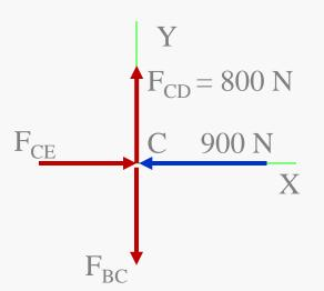
Analyzing pin C:  $\rightarrow + \sum F_X = F_{CE} - 900 = 0$   $F_{CE} = 900 \text{ N} = 0.90 \text{ kN (C)}$   $\uparrow + \sum F_Y = 800 - F_{BC} = 0$  $F_{BC} = 800 \text{ N} = 0.80 \text{ kN (T)}$
