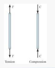
With these two assumptions, the members act as two-force members. They are loaded in either tension or compression. Often compressive members are made thicker to prevent buckling.
