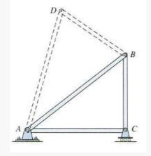
A *simple truss* is a planar truss which begins with a *triangular* element and can be expanded by adding two members and a joint. For these trusses, the number of members (M) and the number of joints (J) are related by the equation M = 2J - 3.
