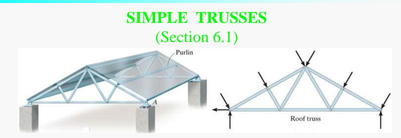
A *truss* is a structure composed of slender members joined together at their end points.
