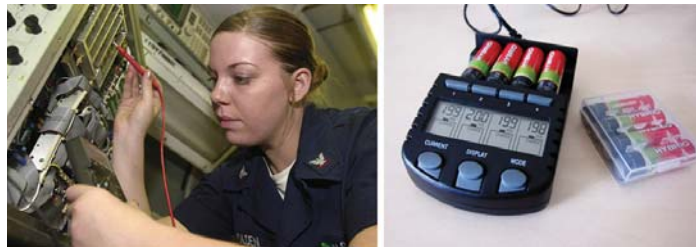
Figure 12.13 These two battery testers measure terminal voltage under a load to determine the condition of a battery. The large device is being used by a U.S. Navy electronics technician to test large batteries aboard the aircraft carrier USS Nimitz and has a small resistance that can dissipate large amounts of power. (credit: U.S. Navy photo by Photographer's Mate Airman Jason A. Johnston) The small device is used on small batteries and has a digital display to indicate the acceptability of their terminal voltage. (credit: Keith Williamson)
