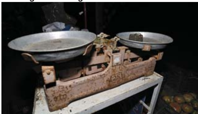
Figure 1.12 A double-pan mechanical balance is used to compare different masses. Usually an object with unknown mass is placed in one pan and objects of known mass are placed in the other pan. When the bar that connects the two pans is horizontal, then the masses in both pans are equal. The “known masses” are typically metal cylinders of standard mass such as 1 gram, 10 grams, and 100 grams. (credit: Serge Melki)
