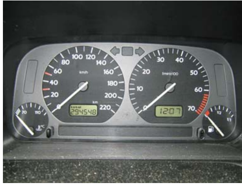
Figure 12.21 The fuel and temperature gauges (far right and far left, respectively) in this 1996 Volkswagen are voltmeters that register the voltage output of “sender” units, which are hopefully proportional to the amount of gasoline in the tank and the engine temperature. (credit: Christian Giersing)
