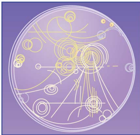
Figure 13.19 Trails of bubbles are produced by high-energy charged particles moving through the superheated liquid hydrogen in this artist's rendition of a bubble chamber. There is a strong magnetic field perpendicular to the page that causes the curved paths of the particles. The radius of the path can be used to find the mass, charge, and energy of the particle.
