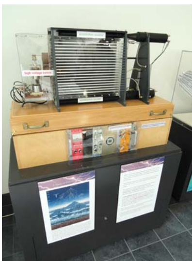
Figure 10.6 A spark chamber is used to trace the paths of high-energy particles. Ionization created by the particles as they pass through the gas between the plates allows a spark to jump. The sparks are perpendicular to the plates, following electric field lines between them. The potential difference between adjacent plates is not high enough to cause sparks without the ionization produced by particles from accelerator experiments (or cosmic rays). (credit: Daderot, Wikimedia Commons)
