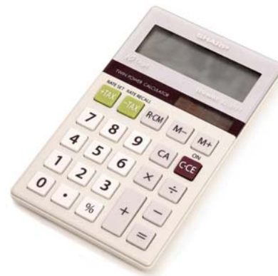
Figure 11.19 The strip of solar cells just above the keys of this calculator convert light to electricity to supply its energy needs. (credit: Evan-Amos, Wikimedia Commons)
