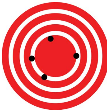
Figure 1.14 A GPS system attempts to locate a restaurant at the center of the bull's-eye. The black dots represent each attempt to pinpoint the location of the restaurant. The dots are spread out quite far apart from one another, indicating low precision, but they are each rather close to the actual location of the restaurant, indicating high accuracy. (credit: Dark Evil)
