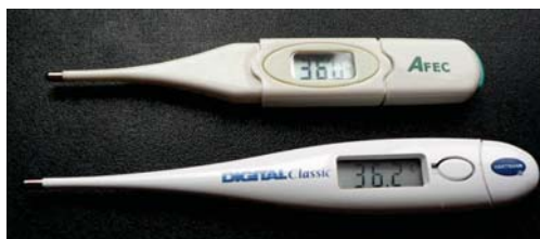
Figure 11.13 These familiar thermometers are based on the automated measurement of a thermistor's temperature-dependent resistance. (credit: Biol, Wikimedia Commons)
