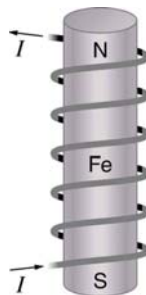
Figure 13.11 An electromagnet with a ferromagnetic core can produce very strong magnetic effects. Alignment of domains in the core produces a magnet, the poles of which are aligned with the electromagnet.
