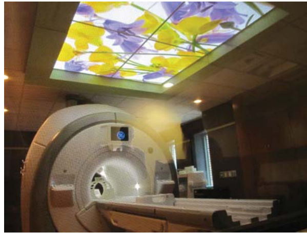
Figure 13.9 Instrument for magnetic resonance imaging (MRI). The device uses a superconducting cylindrical coil for the main magnetic field. The patient goes into this “tunnel” on the gurney. (credit: Bill McChesney, Flickr)
