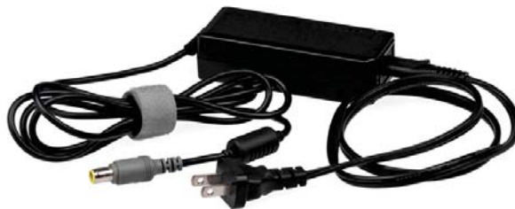
Figure 9.11 This power adapter uses metal wires and connectors to conduct electricity from the wall socket to a laptop computer. The conducting wires allow electrons to move freely through the cables, which are shielded by rubber and plastic. These materials act as insulators that don't allow electric charge to escape outward. (credit: Evan-Amos, Wikimedia Commons)
