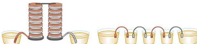
Figure 12.16 Batteries are multiple connections of individual cells, as shown in this modern rendition of an old print. Single cells, such as AA or C cells, are commonly called batteries, although this is technically incorrect.
