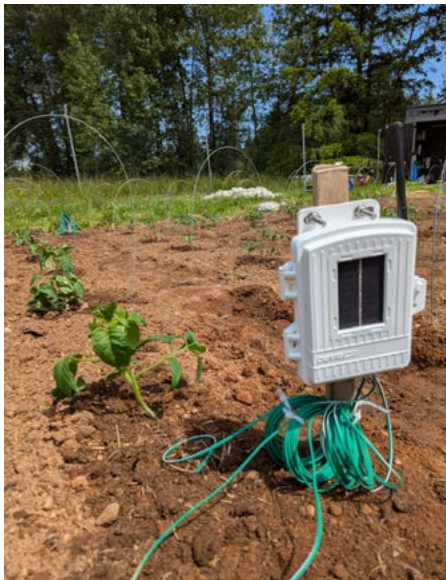
In-ground sensors monitored changes in soil moisture at 1ft, 2ft, 3ft and 4ft depths
