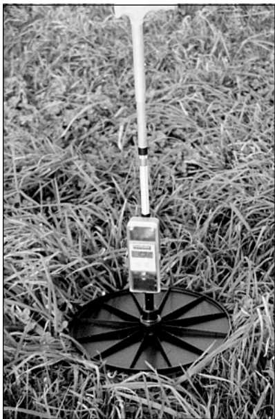
Figure 2.—The electronic rising plate meter estimates standing forage dry matter, accounting for pasture height and density.
