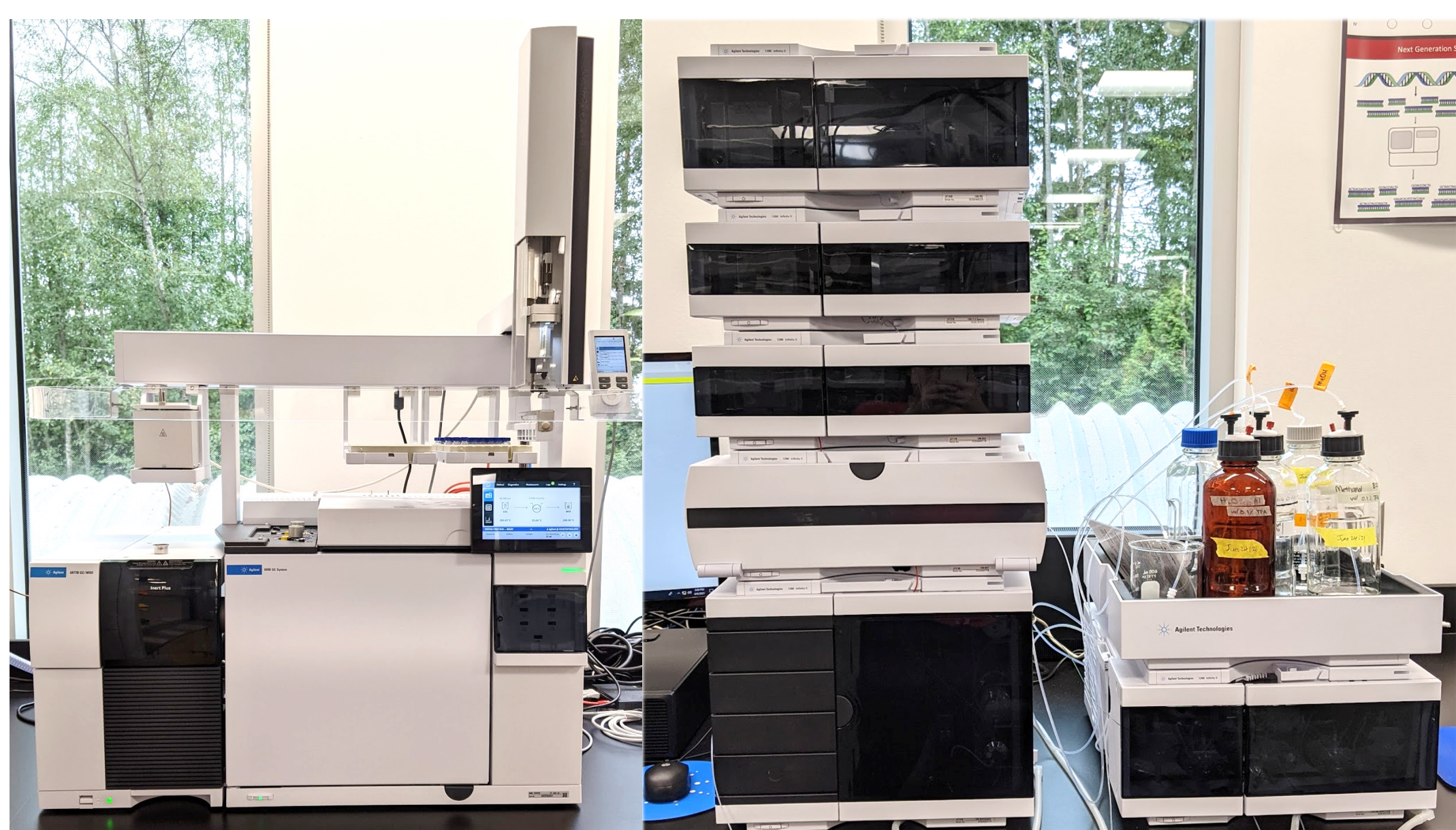
Figure 3. GC-MS (left) and HPLC (right) systems in the AGC lab for chemical analysis in hops cones and leaves.
