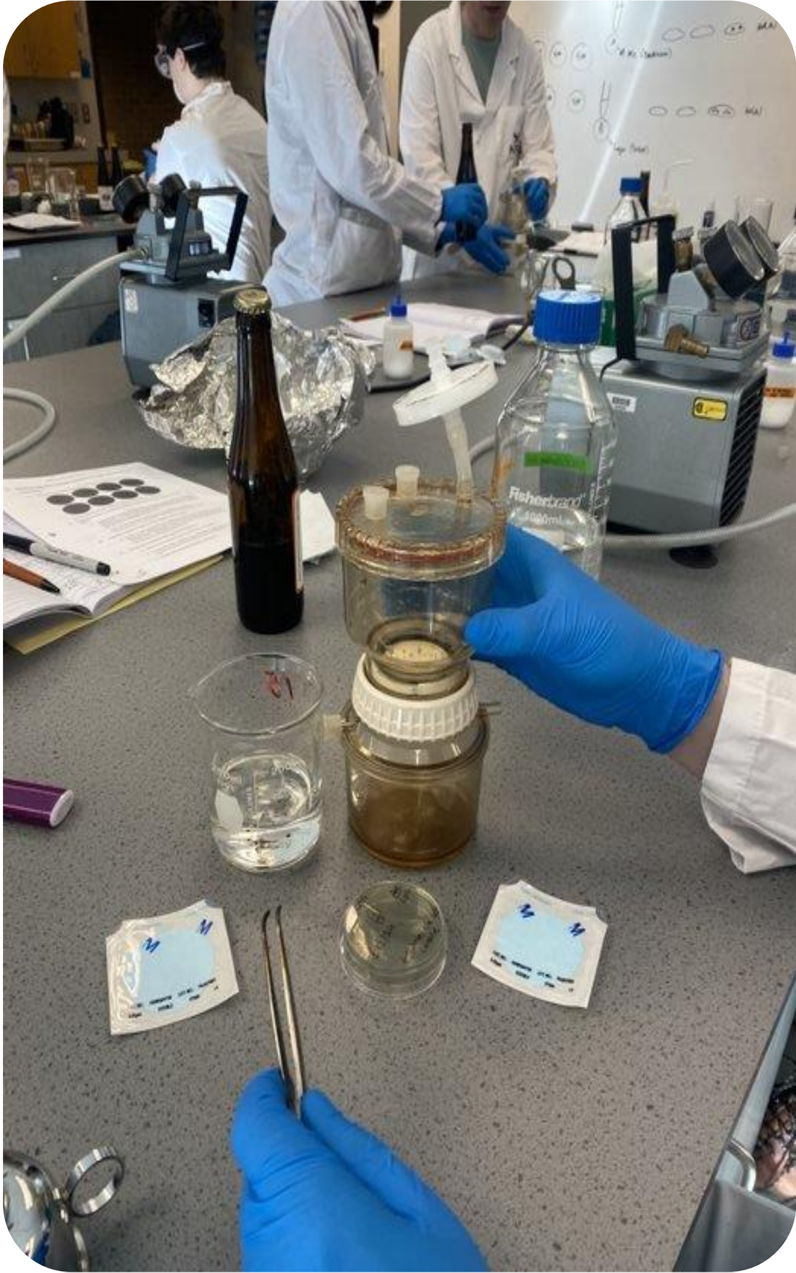
Figure 1: vacuum membrane filter used during plating of bottled pasteurized beer
