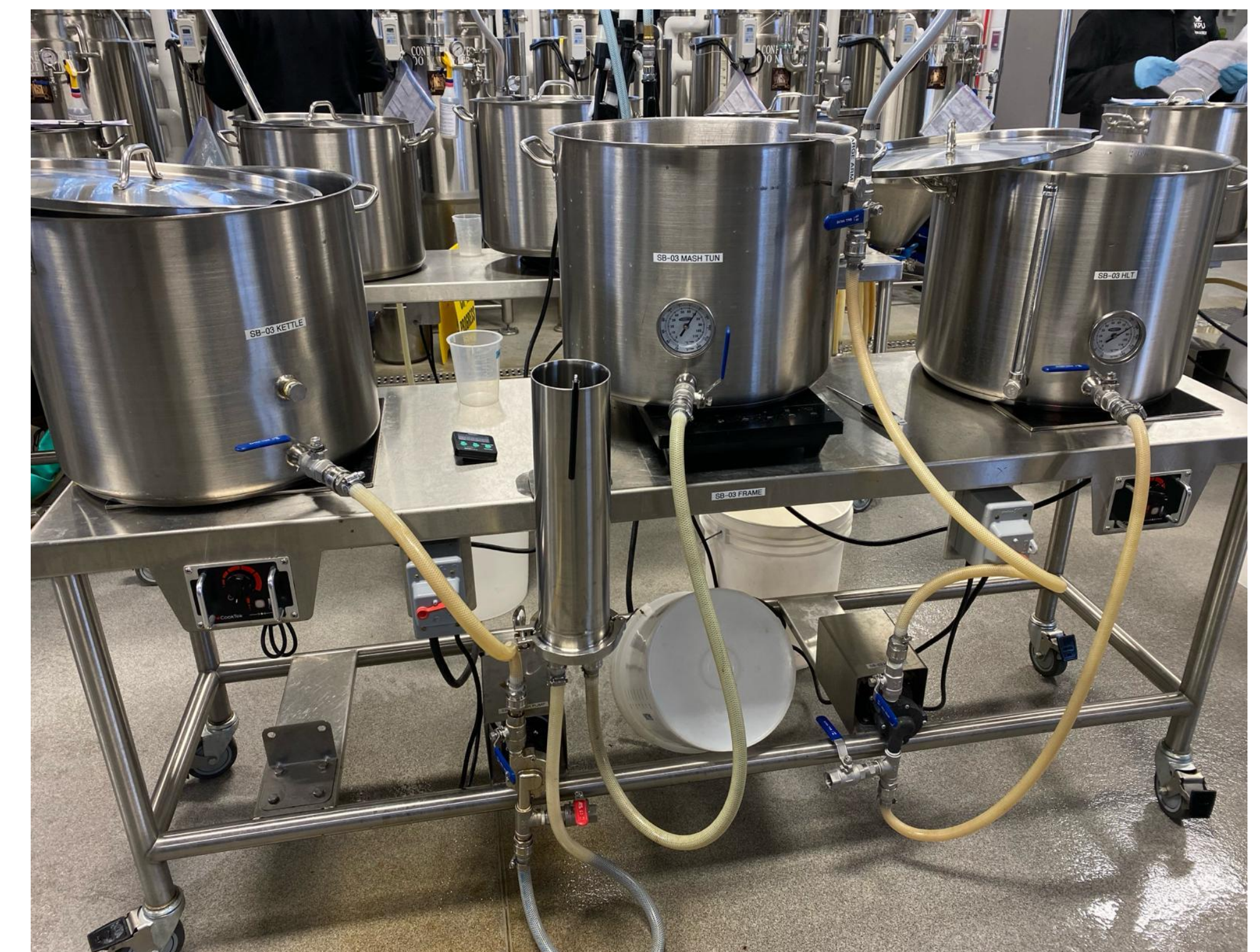
Figure 1.3 Small brewing system (SBS) set up for lautering
